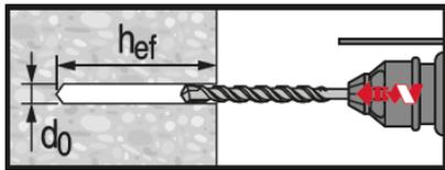
Hammer drilled hole (HD)
