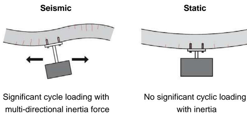
**Figure 7 - Comparison of loading characteristics under seismic and static conditions**
