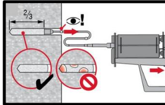
**Injection method** for drill hole depth
