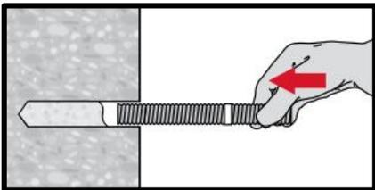
**Setting element**, observe working time " $t_{work}$ ".
