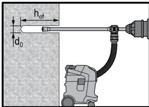
Hammer drilled hole with Hollow Drilled Bit (HDB)
