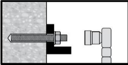
**Loading the anchor:** After required curing time  $t_{cure}$
