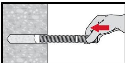
**Setting element, observe working time "t<sub>work</sub>".**
