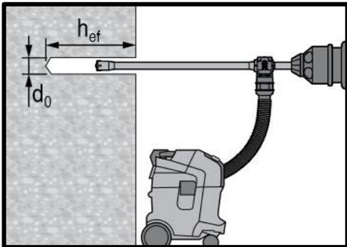
**Hammer drilled hole with Hollow Drill Bit (HDB)**
