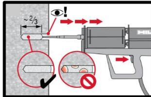
**Injection method** for drill hole depth  $h_{ef} \leq 250$  mm.
