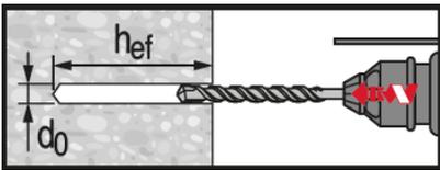
**Hammer drilled hole (HD)**
