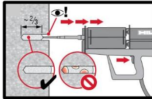
**Injection method** for drill hole depth
