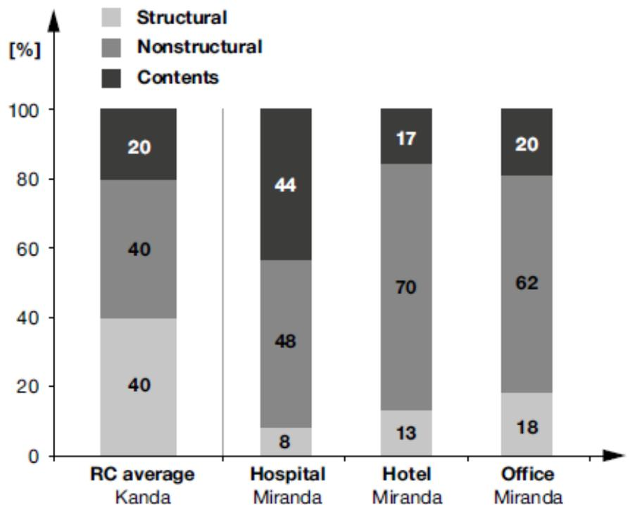
**Figure 1- Repair cost resulting from a seismic event:**
