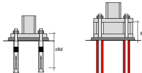
Due to the complexity of defining loads for capacity design and the extreme difficulty of achieving ductile anchor failure in the application, the elastic design approach is often used for base plate application design.
