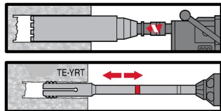
**Diamond Drilling + Roughening Tool (DD+RT)**
