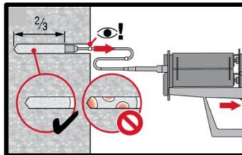
**Injection method** for drill hole depth  $h_{ef} > 250$  mm.
