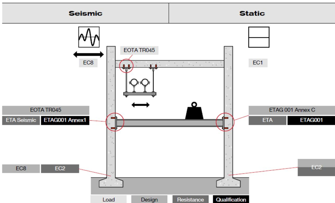
Figure 12 – Overview of the European code system for concrete and anchors
