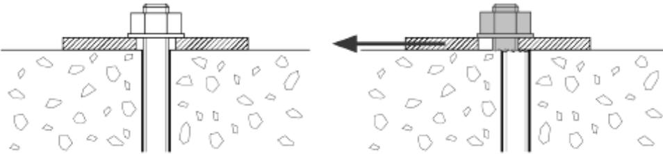
Figure 14 – The possible consequence of an annular gap
