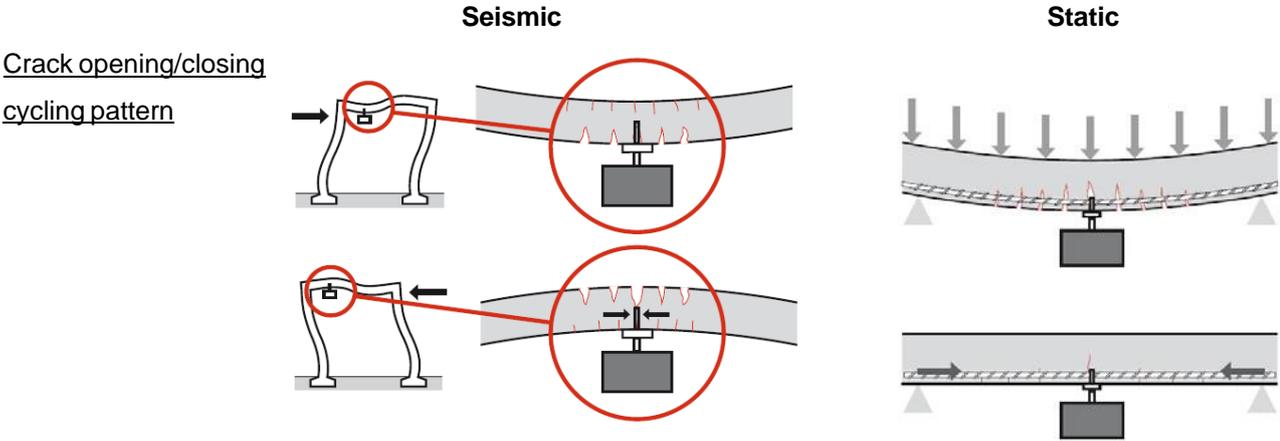
Concrete beside the cracks is alternately under compression and tension, resulting in the worst conditions for the anchor zone.
