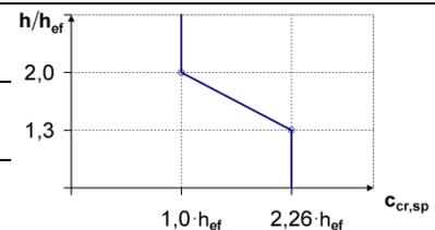
For spacing (edge distance) smaller than critical spacing (critical edge distance) the design loads have to be reduced.
