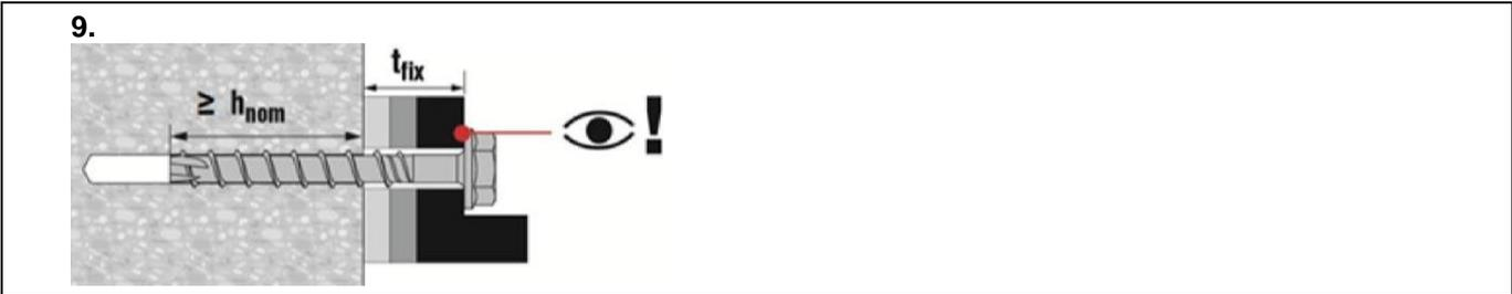
The anchor can be adjusted max. two times.
