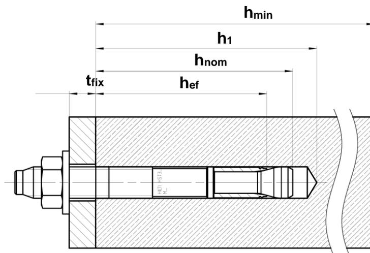
**Setting parameters for M8, M10, M12, M16 and concrete class C20/25 to C50/60**
