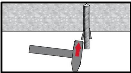
**Setting element for overhead applications**, observe working time " $t_{work}$ ".
