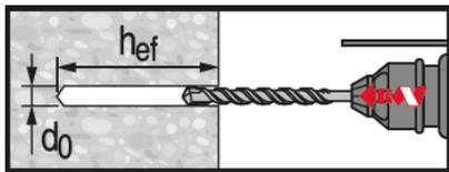
**Hammer drilled hole (HD)**
