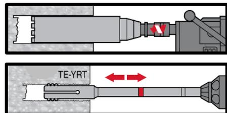
Diamond Drilling + Roughening Tool (DD+RT)
