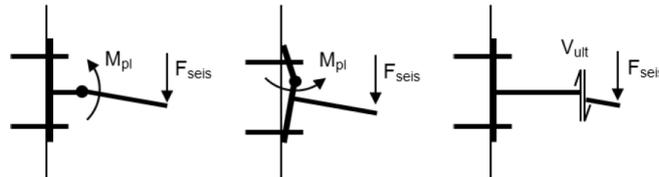
In this case, the load used to design the anchor shall result from the resistance of the attached elements or fixture. However, it is normally very difficult to find the most critical load combination for the anchor group based on the selected elements. It is also not easy to determine the load at which the fixture will yield. This option is therefore most often used in applications where a weak point such as a hinge or rubber is present, the resistance of which can be easily obtained.
