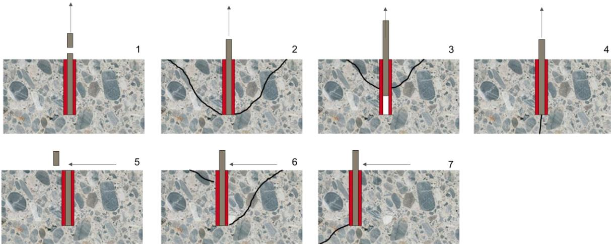
**Figure 11 - Failure modes**
