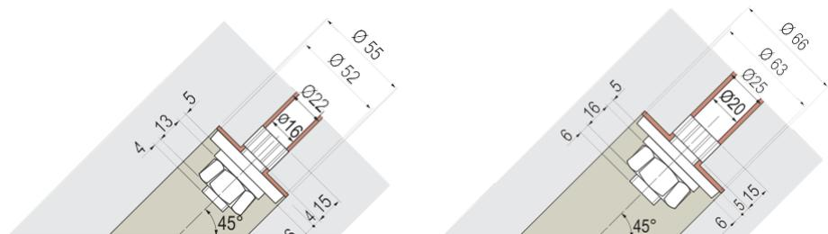
Fig. 32 Anchor head and hole extension HZA-P M16 (left) and M20 (right)
