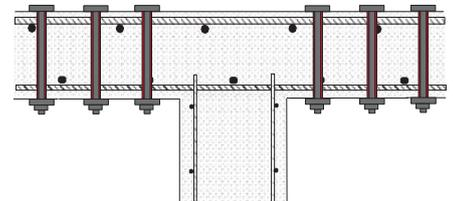
Fig. 1 Penetrating post-installed punching shear reinforcement
