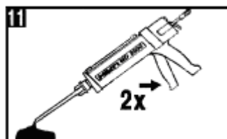
11 Open the HIT-HY 150 resin and "waste" the first 2 trigger pulls.
